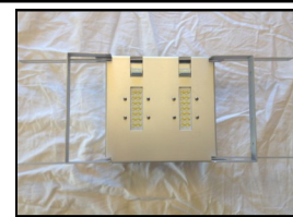
Image 6 – Reattached Brackets/Light Source 90° Orientation
